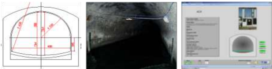
Technical drawings, picture and SCADA screenshot of one of permanent flow sites on Prague sewer network.
