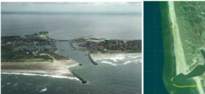
Present breakwater configuration of Hvide Sande harbour (left) and proposed breakwater configuration (right) with the new shoreline (dotted line).
